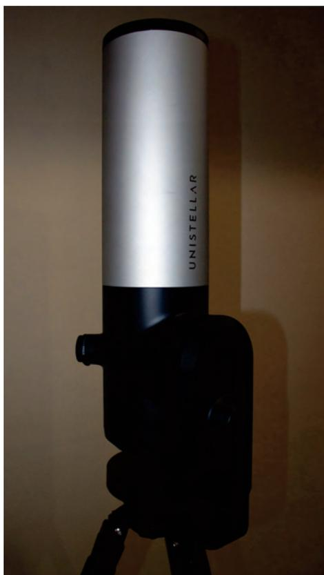
Image 8 - The viewing port near the bottom of the telescope contains a Nikon OLED microviewing screen.
