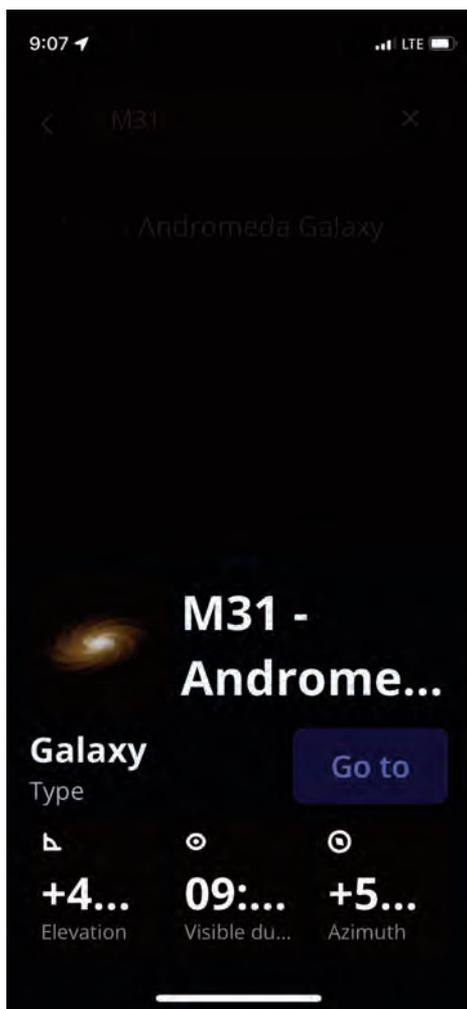
**Image 18** - Once an object is selected, some information on the object is displayed. The telescope will start searching for the object upon pressing the Go To button.
