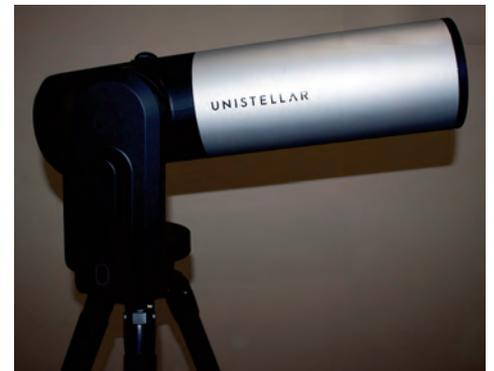
**Image 1 - The Unistellar eVscope 2 is a 114mm f/4 Newtonian with built-in 4.09 megapixel Sony IMX 347 camera at the focal point.**
