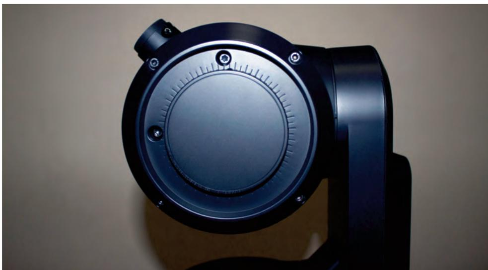
Image 11 - The large spinning knob on the bottom focuses the telescope by moving the primary mirror up or down. It is very easy to focus. There is no image shift during focusing, and the telescope holds the focus quite well!
