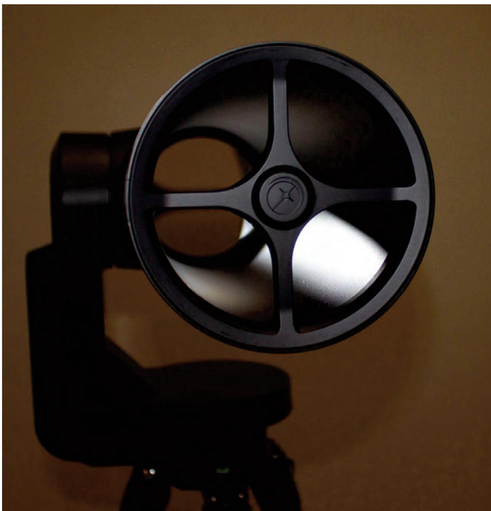
Image 10 - This view shows the 114mm primary mirror. The spider housing contains the Sony camera.
