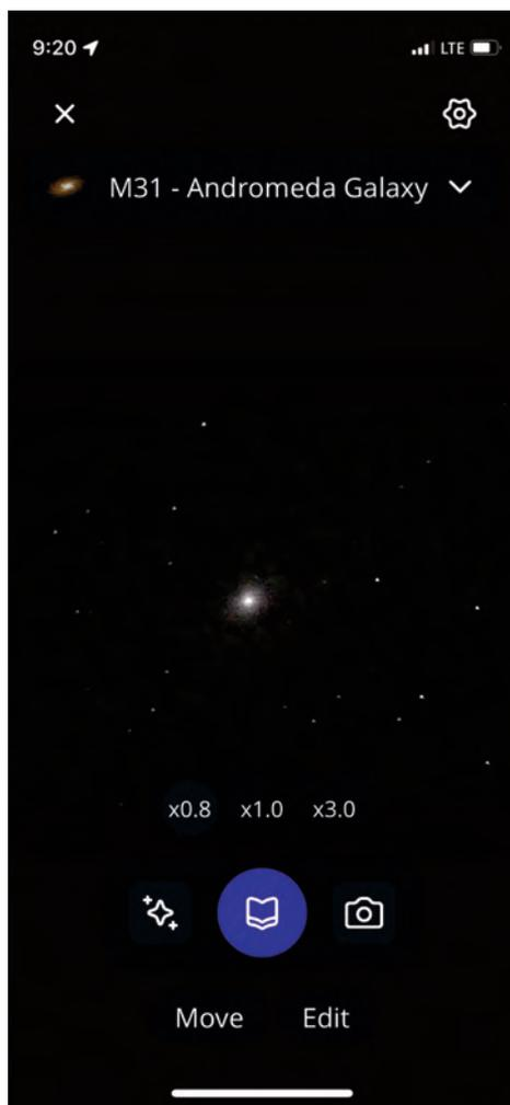
**Image 19** - The telescope will center the object. The user can select viewing it at three different magnifications. The button to the left of the purple button will start camera integration of exposures to achieve a more detailed image of the objects. Pressing the camera icon will save the image to the phone's photo library
