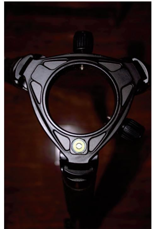
**Image 6 - The tripod top has two hand-turn locking bolts to firmly hold the telescope to the tripod and a bubble level to ensure the telescope base is flat before loading on the telescope.**
